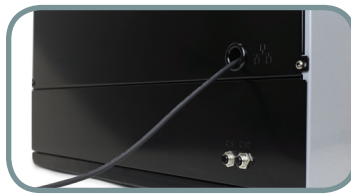
ETHERNET CABLE ROUTING HOLE IN BACK WALL
