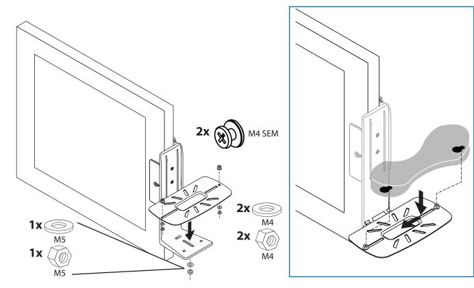
Single hole, center mount: scanner base attaches directly to the L-bracket using: 1 screw, washer and nut.
