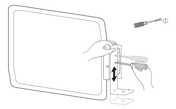
4-corner mount: attach interface plate to L-bracket using 1 washer and 1 nut, then attach scanner base with 4 phillips screws, 4 washers and 4 nuts.
