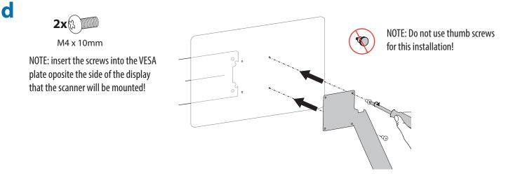
Attach part "1A" to VESA plate at the back of your display. Insert two of the provided M4x14mm phillips screws through the bracket, the VESA plate and display.
