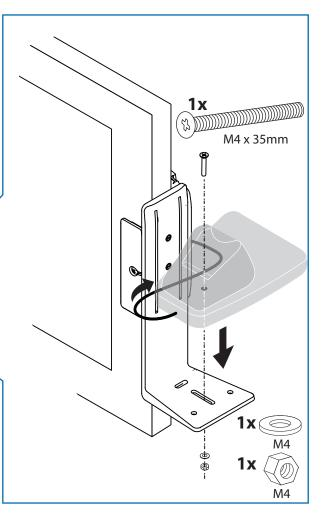
Single hole, center mount plus side screw: scanner base attaches directly to the L-bracket using: 1 screw from bottom, 1 screw from top with washer and nut.
