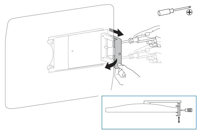
Tighten the front screw until the spacer holds the display snug.
