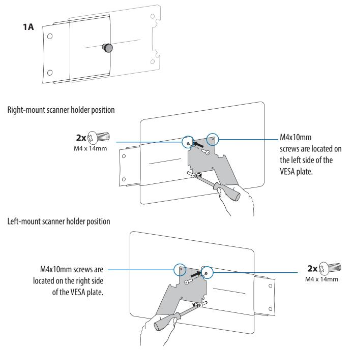
3 Loosen the thumb screw on part "1A" (at the back of the display) and adjust so that part "1B" can be attached to part "1A", then attach "1B" to "1A".
