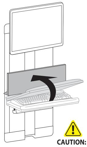
Product is shipped with a stop screw that MUST be removed before use. DO NOT REMOVE STOP SCREW BEFORE ATTACHING KEYBOARD TRAY. Failure too follow these instructions will cause equipment damage.
