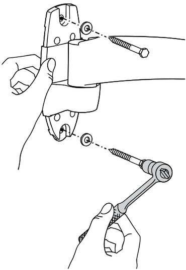
**CAUTION:** Make sure the wall mount bracket is level, flush and snug to the wall surface.
