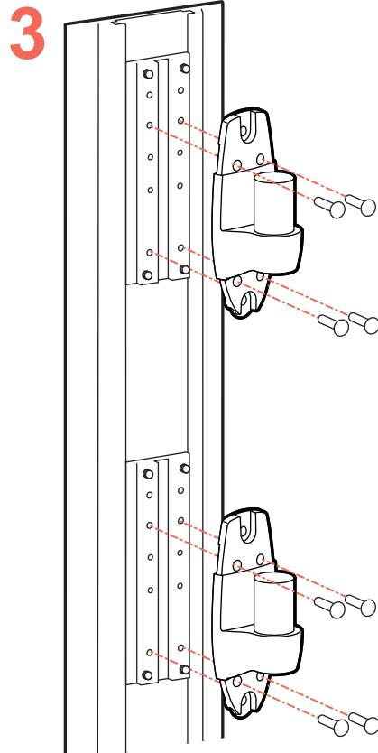
**EN** NOTE: Fasteners may unwind due to vibration caused by movement of mounting solution over time. Inspect mounting solution for loose fasteners on a routine basis. If desired, apply a light duty thread locking adhesive to fasteners before installation to prevent back-out.
