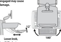
Loosen knob, tilt Display to desired position then retighten knob.
